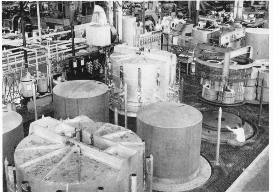
Truspec Aluminum Coils ready for annealing are loaded on the furnace platforms. The unique feature of these new furnaces is that separate devices are placed over the bases by a crane as required during the annealing cycle.
